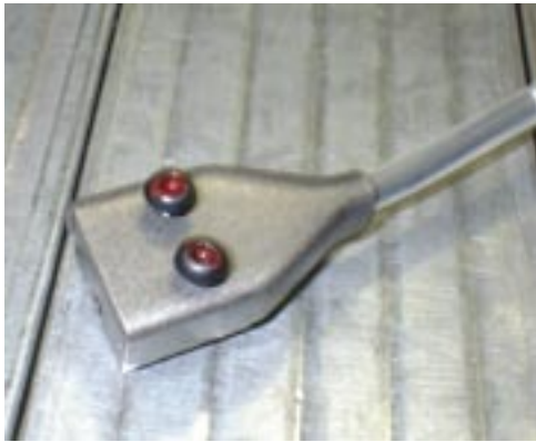
Electronic solid-state switch with PNP outputs. NPN outputs available on request
