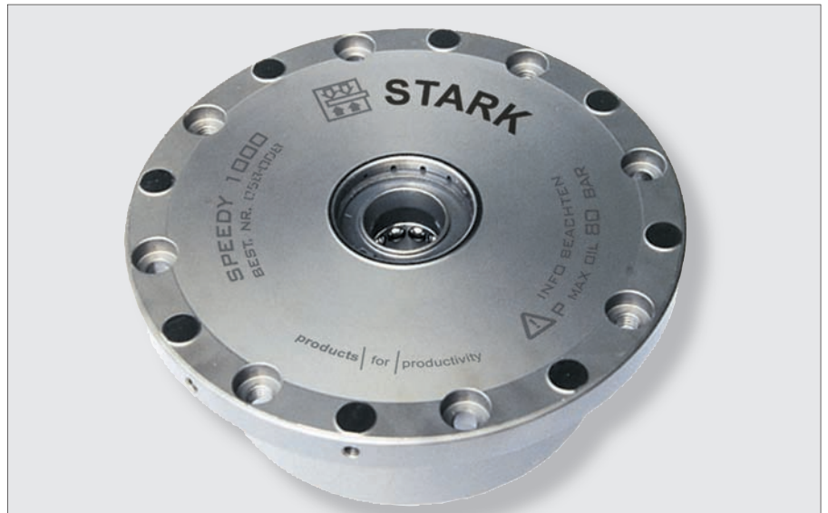
SPEEDY classic - clamps mechanically and releases hydraulically
