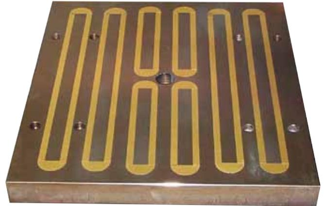
M-TECS 240 opens up brand new paths for the rubber and the duroplastics processing industries. With no downtime or waiting time to cool down or heat up tools, retooling times can sometimes be cut by hours. Using the advanced magnetic clamping technique, moulds can be changed even when they are hot as the operator will not make contact with them at all. This is both convenient and safe.
