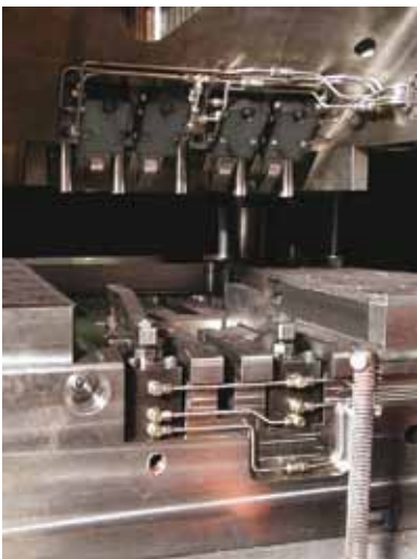
Use of wedge clamps with sequence valve control in a forging press
