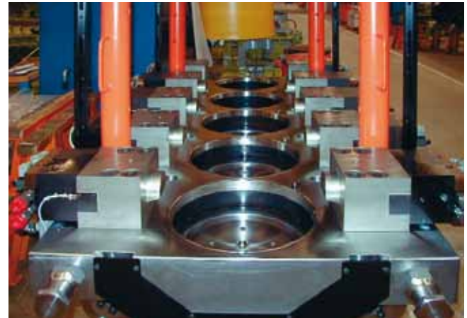
5-stage drop forging press equipped with wedge clamps with directional seat valves to activate the different stages
