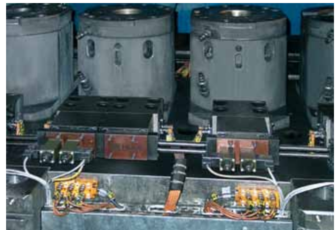
Wedge clamps with flanged directional seat valves. Clamping and unclamping positions are electrically controlled. Little installation work as a result of plug-type connections between the clamps.
