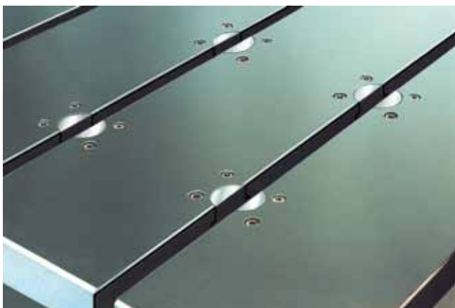
Pull clamping elements with T-slot installed in a press bed
