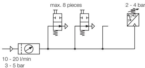
For the evaluation of the pneumatic pressure built-up standard pneumatic pressure switches can be used. It is possible to control with one pressure switch up to 8 position monitorings connected in series (see circuit diagram). It has to be considered that process-safe functioning of pneumatic position monitorings is only guaranteed with throttled air and system pressure. The nominal values are indicated below technical characteristics.
