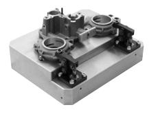
Options for clamping levers Clamping lever with swivel contact bolt
