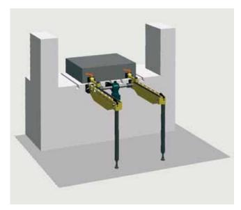
Roller and ball bars in the T-slots of the table provide for easy insertion of the die, either manually or automatically. Damage to the die causing production loss is avoided. Individual solutions including automatic die changing and integration in the press are possible.
