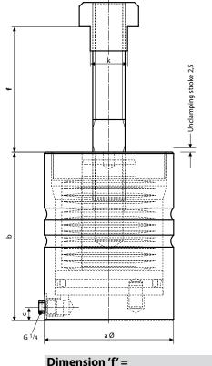
die clamping edge + web height + unclamping stroke
