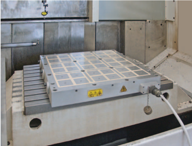
Magnetic clamping plate with square poles 70 x 70 mm, plate size 630 x 630 mm with lateral bore holes for stop bars
