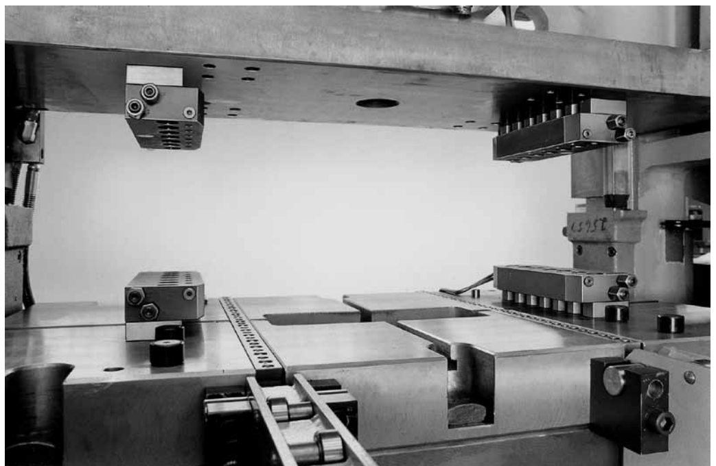
Clamping bars installed in press bed and ram. Easy loading of dies using die change consoles and lateral guide rollers.
