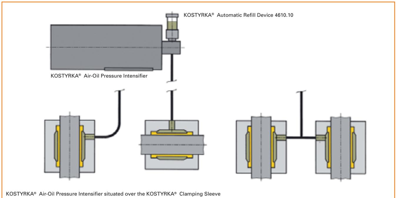
If the pressure intensifier is fitted **under** the clamping sleeve, the automatic refill device must be separated from the intensifier. The pressure line is best taken to the lowest point of the installation space and on from its uppermost
