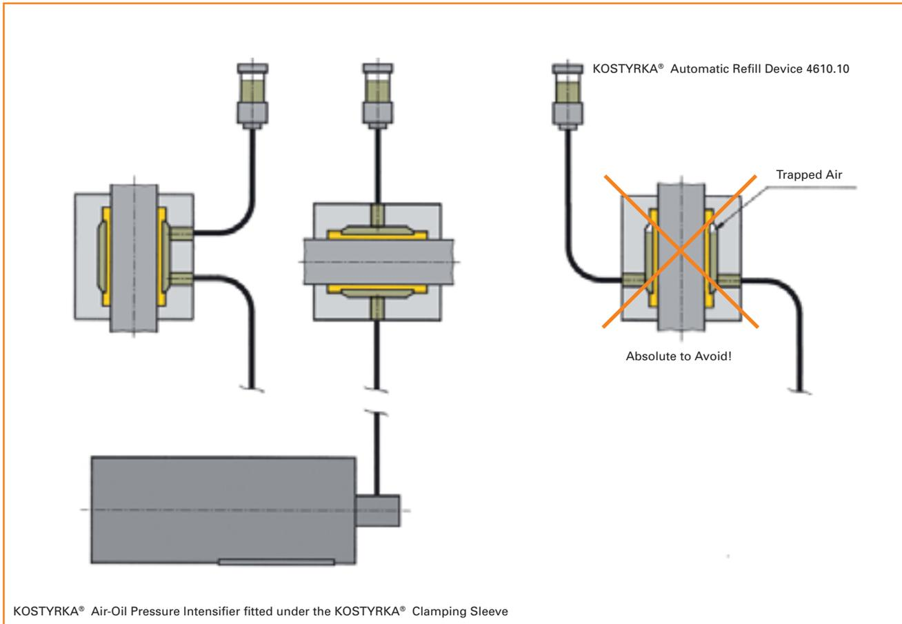
KOSTYRKA® Air-Oil Pressure Intensifier fitted under the KOSTYRKA® Clamping Sleeve
