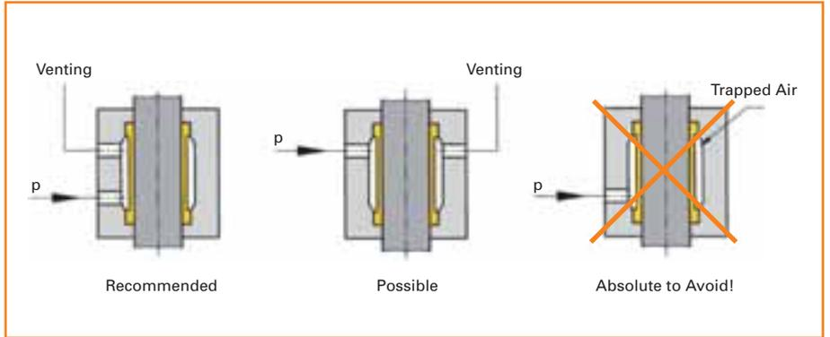
**7.7.2 ...when Mounting the KOSTYRKA® Clamping Sleeve Horizontally**
