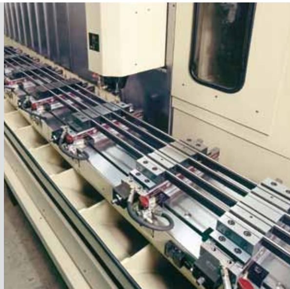
DS hydraulic with floating jaws
