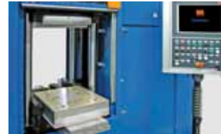
M-TECS 240-G for the rubber and the duroplastics processing industries, temperature resistant up to 240°C
