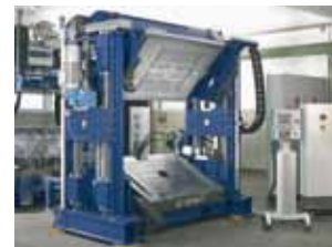
M-TECS 80-F for mould carriers, temperature resistant up to 80°C
