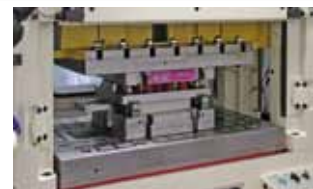
M-TECS 80-B for sheet-metal forming, temperature resistant up to 80°C
