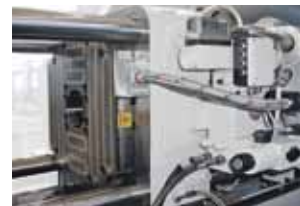
M-TECS 240-D for die casting machines, temperature resistant up to 240 °C
