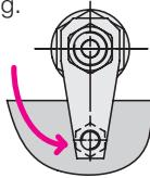
Clamping arms and strap type clamps are fastened to the piston rod by means of a taper shank and socket connection.
