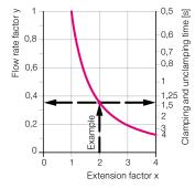
Adm. flow rate and clamping time as a function of the clamping arm extension
