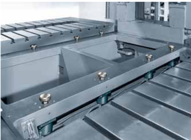
Clamping of a complete die changing table with pull clamping elements.
