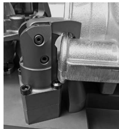
Clamping of a cast part with special clamping lever
