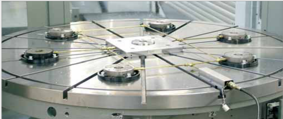
SPEEDY classic 2 Surface Mount with hydraulic pipework
