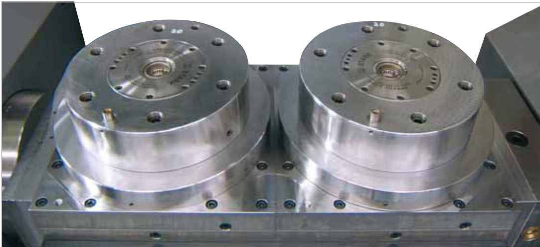
SPEEDY classic 2 with two integrated media ducts, fitted to swivelling yoke.
