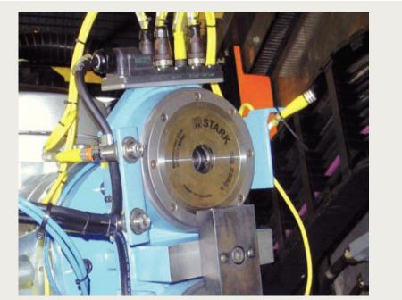
SPEEDY airtec 1 fast closing clamp, built into a robot arm for changing workpieces. Pallet identification and presence check via sensors on the changer arm.
