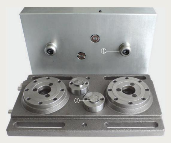
Coupling elements are used for the provision of hydraulic oil and air, other media on request. The coupling element does not require any coupling stroke, can only be coupled de-pressurised. The necessary positioning is ensured together with the SPEEDY airtec fast closing clamp.
