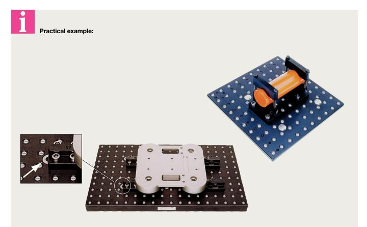
Nipple fastening variant D and E. Makes it possible to manufacture the nipple fastening in one work step. As a result the highest accuracy is achieved.
