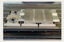
SPEEDY airtec module plate, designed for clamping using 6 fast closing clamps.
