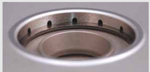
Openings for centre blow-out ducts
