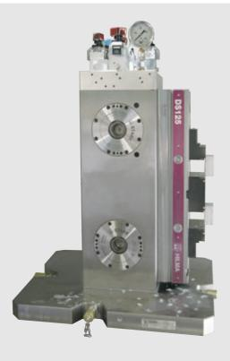
SPEEDY classic 2 fast closing clamps with media ducts fitted to each side of the mounting tower. Machine vices are operated by the control valves fitted at the top.
