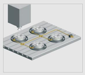
Position fast closing clamps and fasten using the fixing clamps.
