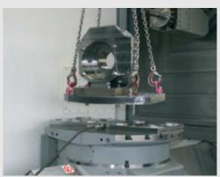
Easy, quick changing of a jig with SPEEDY classic 2, couple, release and lift off. Due to the contour of the retractable nipples, it is also possible to remove asymmetrical jigs at an angle.
