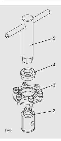
Slide sealing sleeve (2) and valve pin into the bore.
