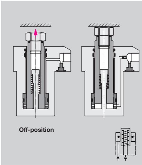
The support plunger contacts the workpiece by air pressure. The contact force is proportional to the air pressure less spring return force.
