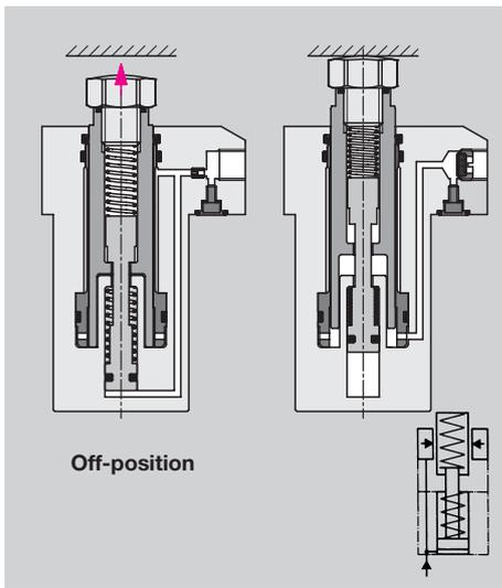
The support plunger is extended by a hydraulically pressurised small piston and contacts the workpiece with spring force.
