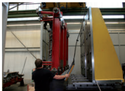
Wotan: machine table with right-angled clamping plate 1 and right-angled clamping plate 2. Loading is undertaken using the overhead crane. The „third hand function“ and optional clamping check are also an advantage during handling like the optical release check.
