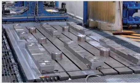
SPEEDY classic 3 fast closing clamps fitted in clamping strips with pipework. Using the two jigs, workpieces up to 12 m can be clam-
