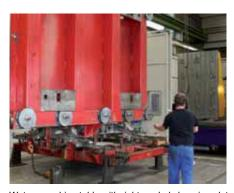
Wotan: machine table with right-angled clamping plate 1 and right-angled clamping plate 2. Loading is undertaken using the overhead crane. The "third hand function" and optional clamping check are also an advantage during handling like the optical release check.
