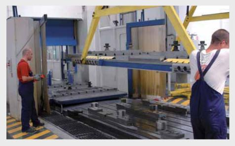
Loading using the handling system manufactured by STARK.
