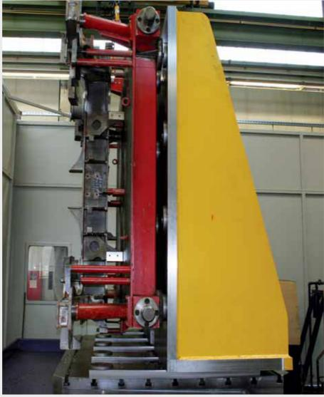
Clamping angle for workpieces up to 2.5 m high with 12 SPEEDY classic 3, 360 kN insertion force.
