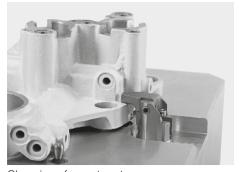
Clamping of a cast part
